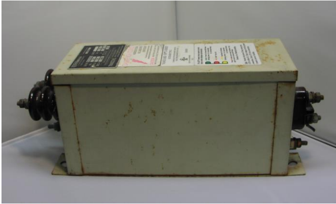
Figure 2-1 -- High voltage power supply (unsafe)
